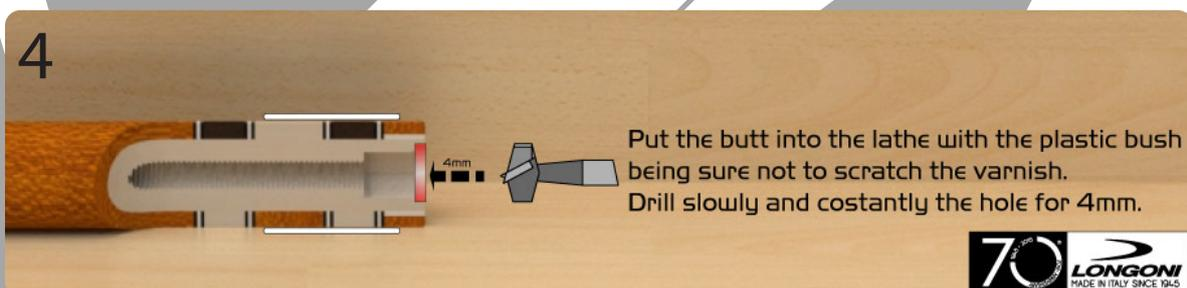
Put the butt into the lathe with the plastic bush being sure not to scratch the varnish. Drill slowly and constantly the hole for 4mm.
