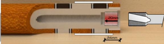
Thread the hole for 20mm, checking that the tool enter straight in the center
