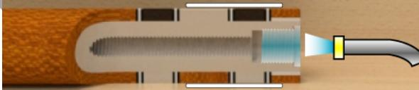
Clean perfectly the hole with compressed air. Check if the 3Lobite component can easily enter till the end by hand without glue.
