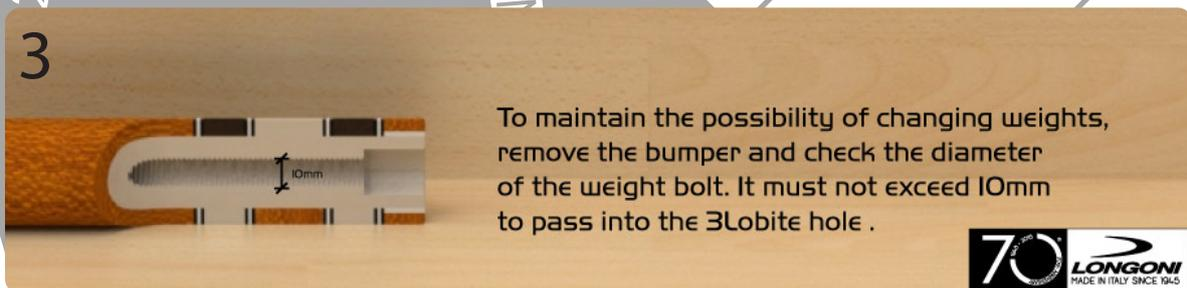
To maintain the possibility of changing weights, remove the bumper and check the diameter of the weight bolt. It must not exceed 10mm to pass into the 3Lobite hole.
